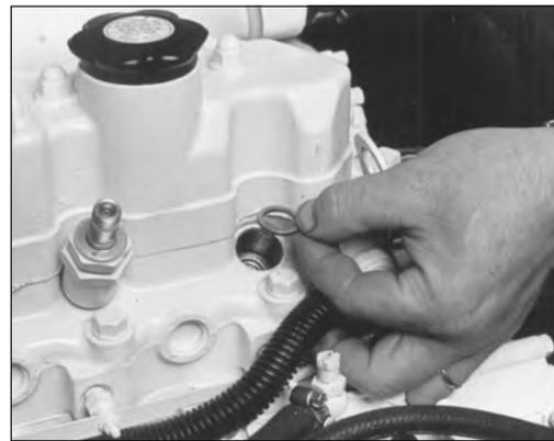
**Figure 12:** Remove and replace copper sealing washer.
