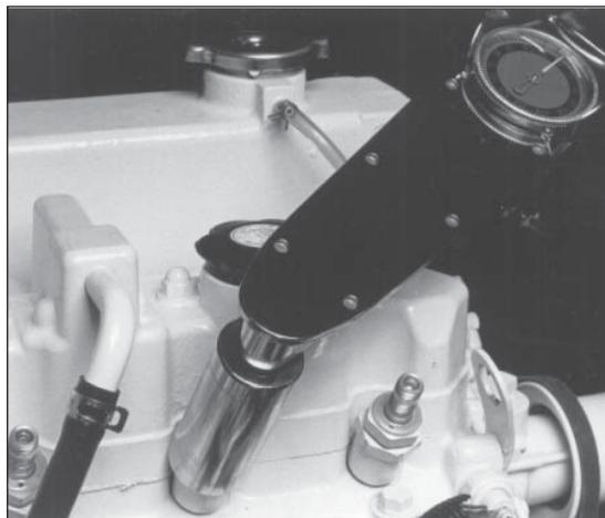
**Figure 18:** Reinstall injector. Torque to proper tightness.
