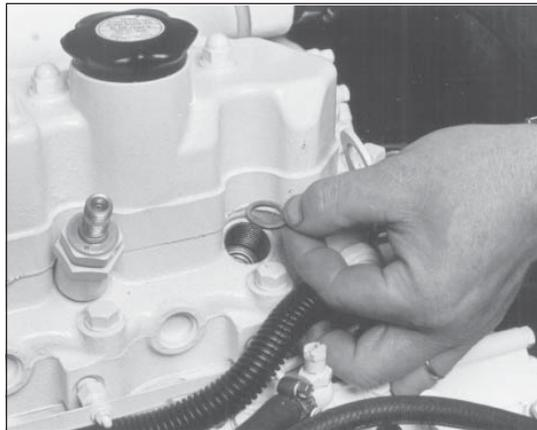
**Figure 17:** Remove and replace copper sealing washer.
