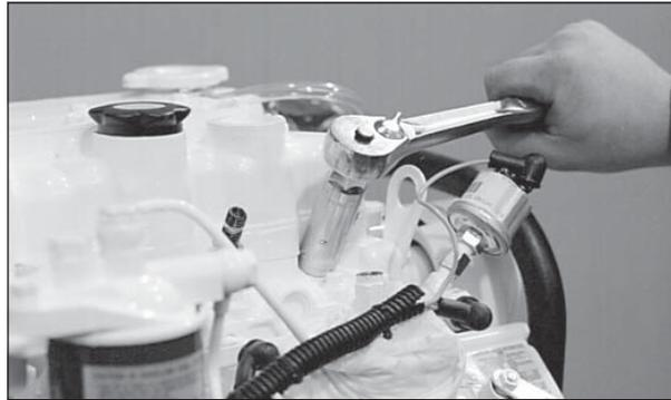
**Figure 18:** Unscrew injector.
