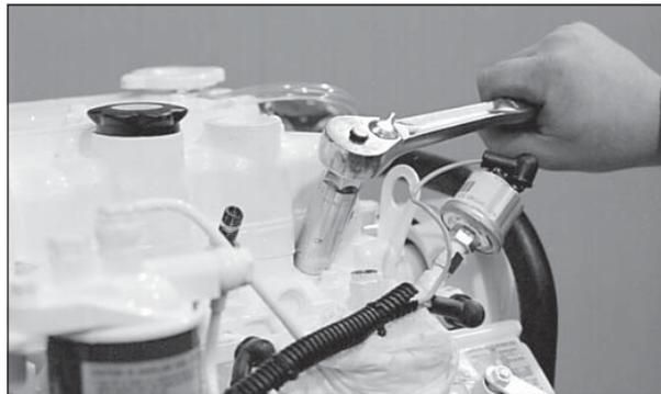
**Figure 17:** Unscrew injector.
