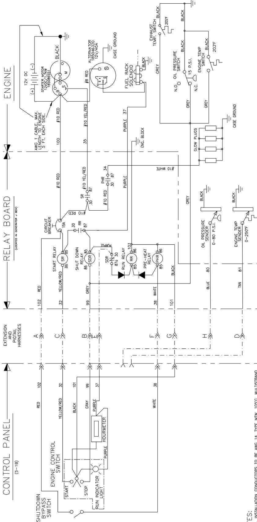
**Engine Wiring Schematic**
