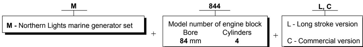
**M844k** = Northern Lights marine diesel generator set with an 844 engine and a PX-300K generator end.
