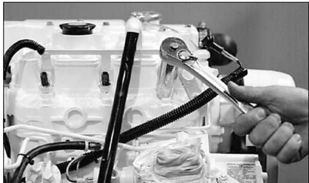
**Figure 16:** Unscrew injector.
