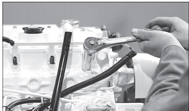
**Figure 17:** Reinstall injector. Torque to proper tightness.
