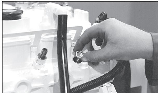
**Figure 16:** Remove and replace copper sealing washer.
