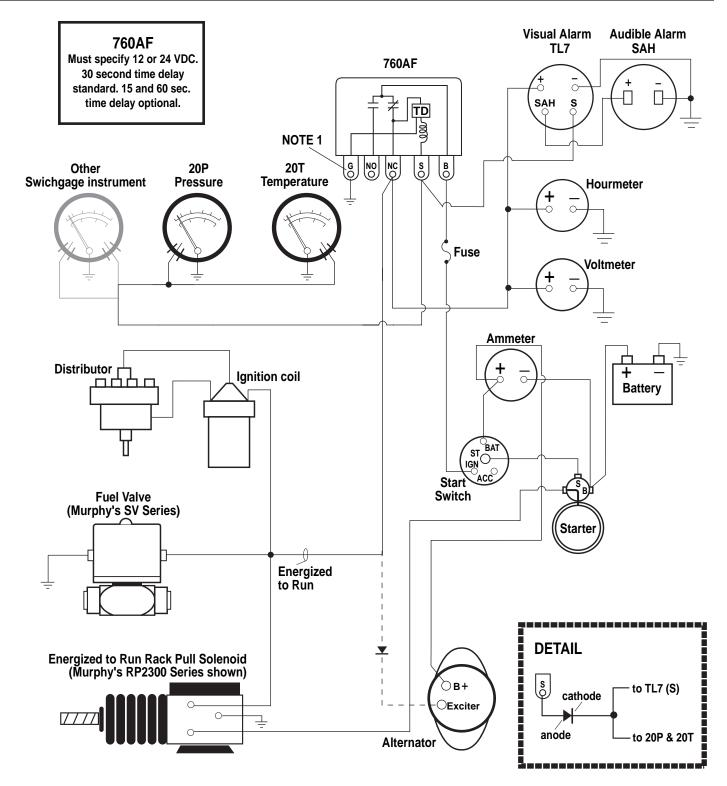
NOTE 1: With 760AF terminal "G" grounded, the time delay operates only on start; after the initial time delay, the shut-down circuit is operated immediately when SWICHGAGE® contact operates.
