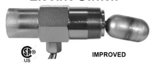
**LS200** Liquid Level Switches with 2" NPT mounting are float activated to operate an electrical SPDT snap switch (optional DPDT on some models) for alarm or shutdown of an engine or electric motor. The LS200 connects directly into the vessel wall and can be used with a Murphy weld collar (P/N 15050375) or Murphy external float chamber (P/N 15700799).
