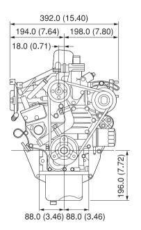
Shown above: with Kubota Standard flywheel and rear-end-plate. Option kit for Clutch No.6 1/2" Flywheel and SAE No.5 Flywheel Housing is also available.
