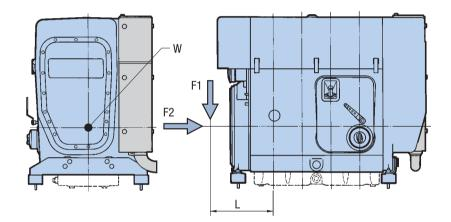
Shaft W: Suitable for axial power-take-off, for example adaption of a hydraulic pump.
