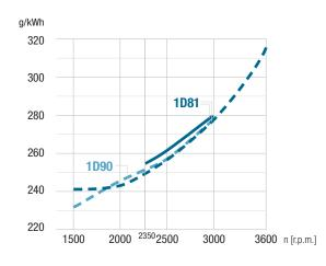
▶ Performance data refer to Standard Reference Conditions of ISO 3046-1: + 25 °C (77 °F), 100 kPa, relative humidity 30 %. During running-in period the output increases by approx. 5 % which is taken into consideration at delivery.
