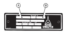
The model type A and the engine serial No. B are given in the engine identification plate.
