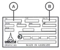
The model type A and the engine serial No. B are given in the engine identification plate.
