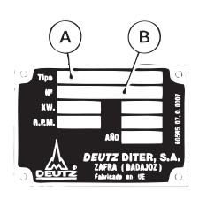
The model type A and the engine serial No. B are given in the engine identification plate.
