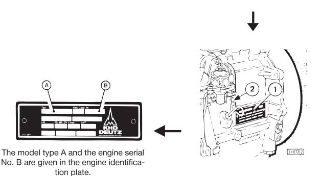
The engine identification plate 1 is mounted to the crankcase.
