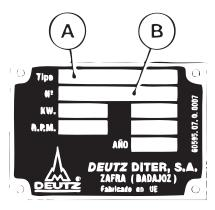
The model type A and the engine serial No. B are given in the engine identification rplate.
