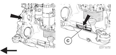
The engine identification plate C is mounted to the crankcase. The serial No. is also stamped into the crankcase.
