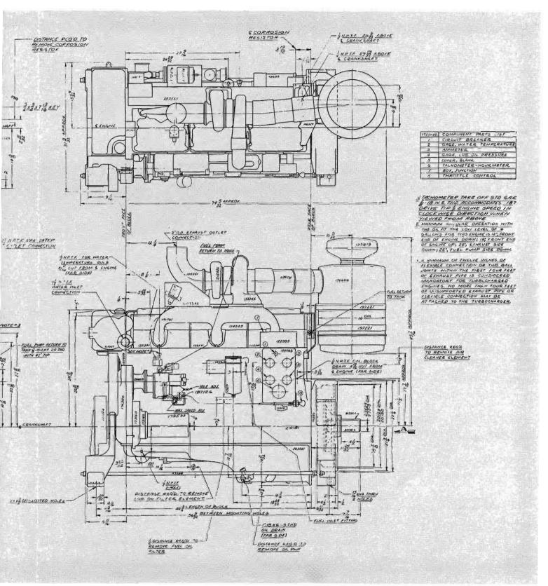
NT-855-F1 Engine Installation Diagram 208359
