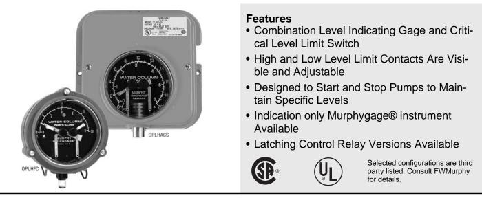
The OPLHC/OPLHACS Series Level Swichgage instruments are combination level indicating gages with adjustable low and high limit switches. Limit switches can be wired directly to electric pilot circuits to operate alarms, shutdown or start/ stop pumps to maintain predetermined levels.
