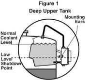
For **MARINE AND MOBILE EQUIPMENT** installations, the top tank connection should be near the vertical centerline of the radiator. This will compensate for changing level due to roll and pitch of the machine during operation.
