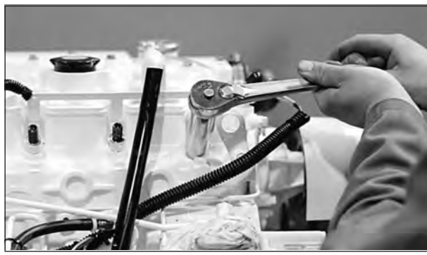
Figure 17: Reinstall injector. Torque to proper tightness.
