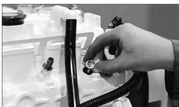
Figure 16: Remove and replace copper sealing washer.
