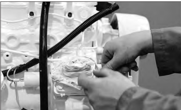
Figure 12: Cover lines, inlets and injection pump outlets.
