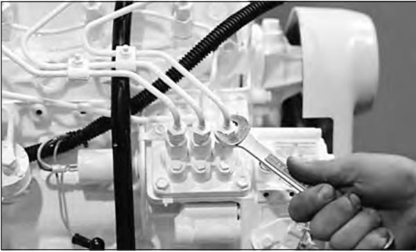
Figure 10: Remove delivery line flare nuts.
