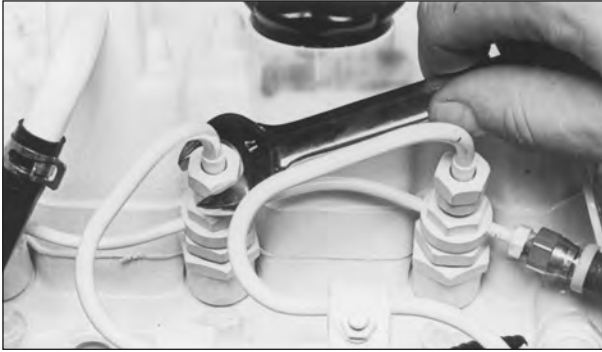
Figure 7: Remove delivery line flare nuts.
