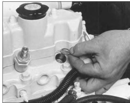
Figure 12: Remove and replace copper sealing washer.
