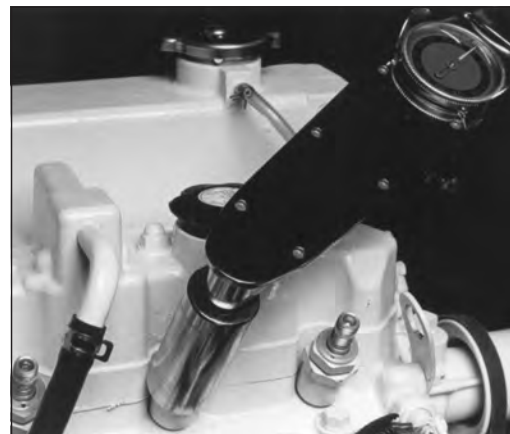
Figure 13: Reinstall injector. Torque to proper tightness.
