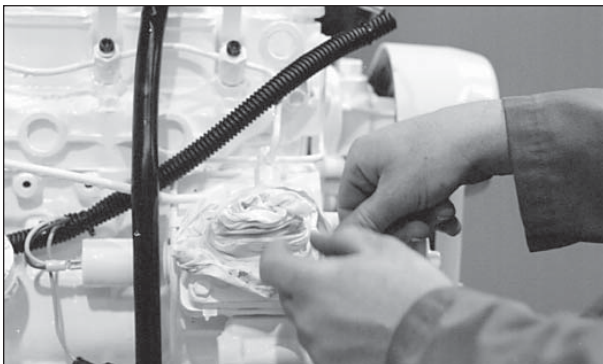
Figure 11: Cover lines, inlets and injection pump outlets.
