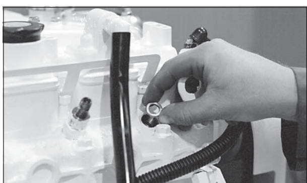
Figure 16: Remove and replace copper sealing washer.
