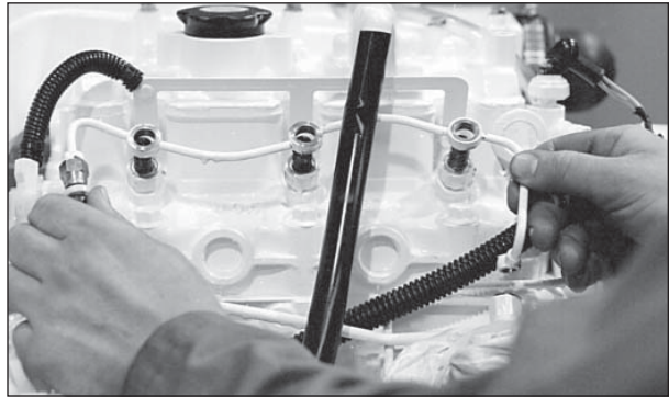
Figure 14: Remove return line.
