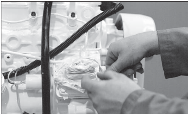
Figure 12: Cover lines, inlets and injection pump outlets.
