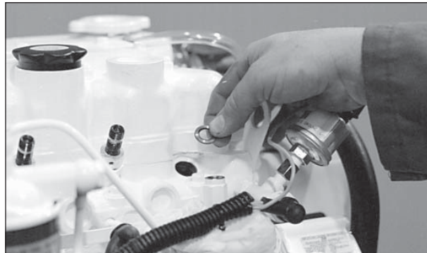
Figure 18: Remove and replace copper sealing washer.
