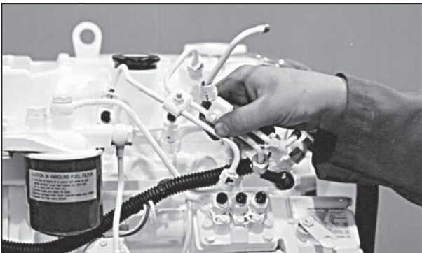
Figure 13: Remove delivery lines.
